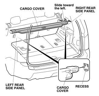
5. Pull out the cargo cover, and attach the right and left rods on the cargo cover to the right and left rear side panel.
